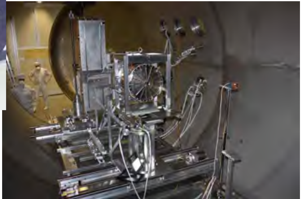
FXT STM Mirror Module at PANTER facility for X-ray tests (credit Media-Lario)
